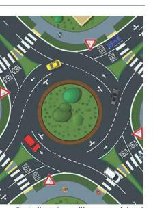
Illustration of a multilane roundabout Source: FHWA
