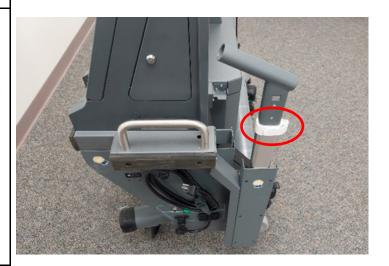
Remove the smaller cap and take the curtain out from tube on the back of the machine.
