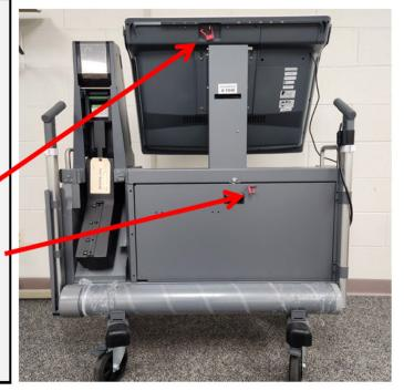
Use the voting machine keys to **open the rear access door** on all voting machines. Remove the surge protectors, extension cords, activation cards, audio headset, and the ADA controller inside.
